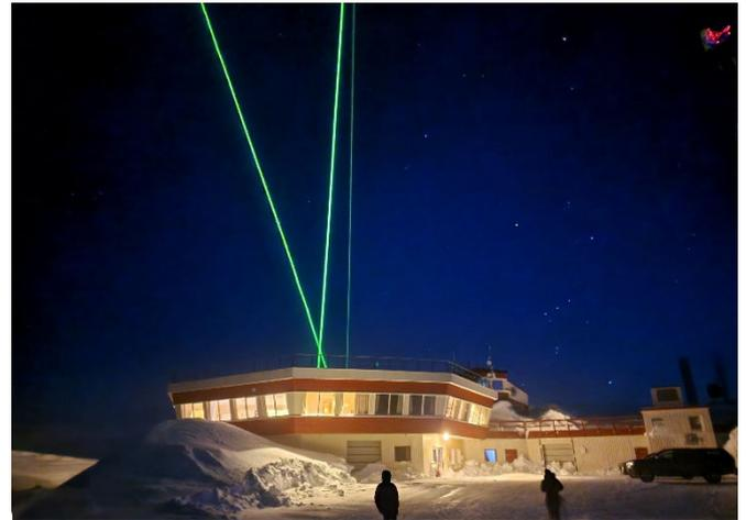
Abbildung: Optical sounding of the atmosphere up to the Edge of Space by Lidar (Light detection and ranging) from Northern Norway
